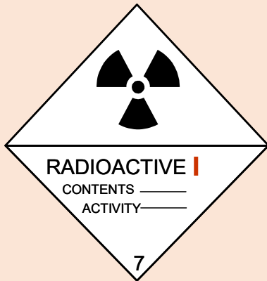
RADIOACTIVE WHITE-I Label: The Entire label has white background, and the 'I' is in red.
