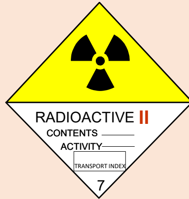
RADIOACTIVE YELLOW - II Label: Top half of the triangle is in yellow, and the 'II' is in red.
