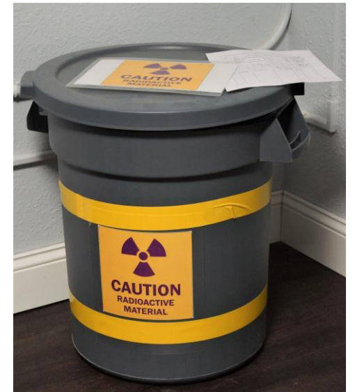
Dedicated radioactive waste receptacle: note waste log on top of container. For temporary / hot lab storage, the container must be lead lined. For long term DIS in a remote area, steel drums may be acceptable
