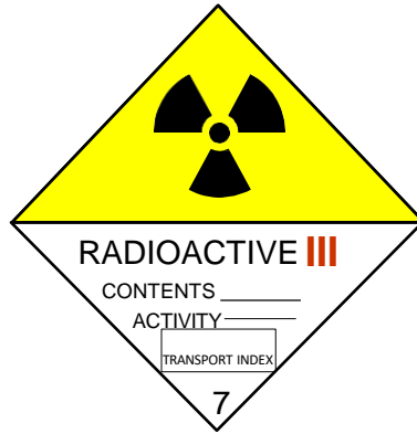
RADIOACTIVE YELLOW - III Label: Top half of the triangle is in yellow, and the 'III' is in red.
