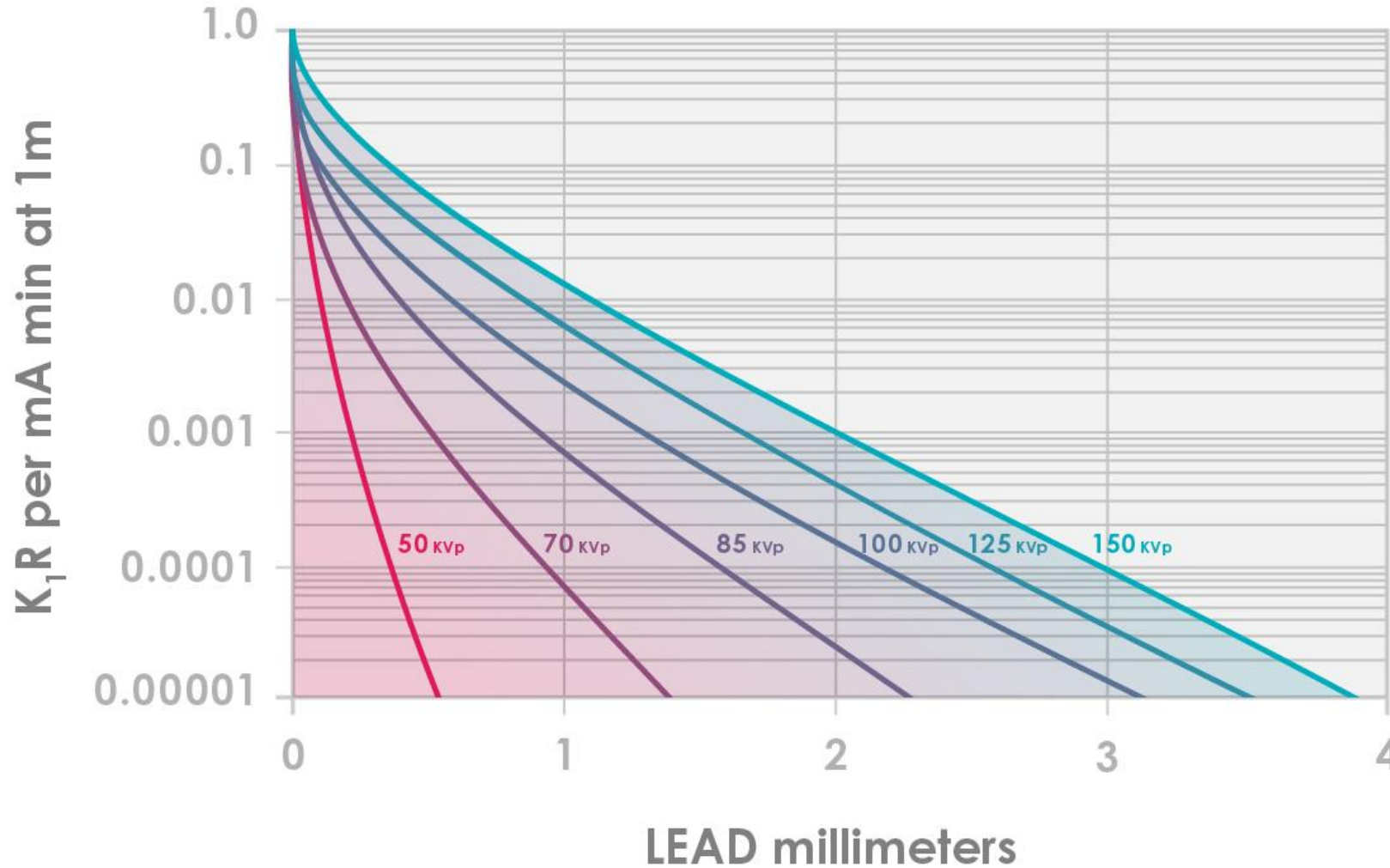
Data chart of lead thickness vs K value for operating voltages from 50 kVp to 150 kVp
