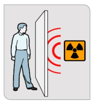
Shielding: If you have a thick shield between yourself and the radioactive materials more of the radiation will be absorbed by the thick shield, and you will be exposed to less.
