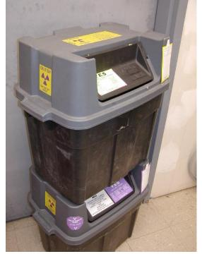
Above is a standard waste container labeled for radioactive waste. The solid waste from <sup>117m</sup>Sn contains such a small amount of radioactivity that the container is not required to be shielded.
