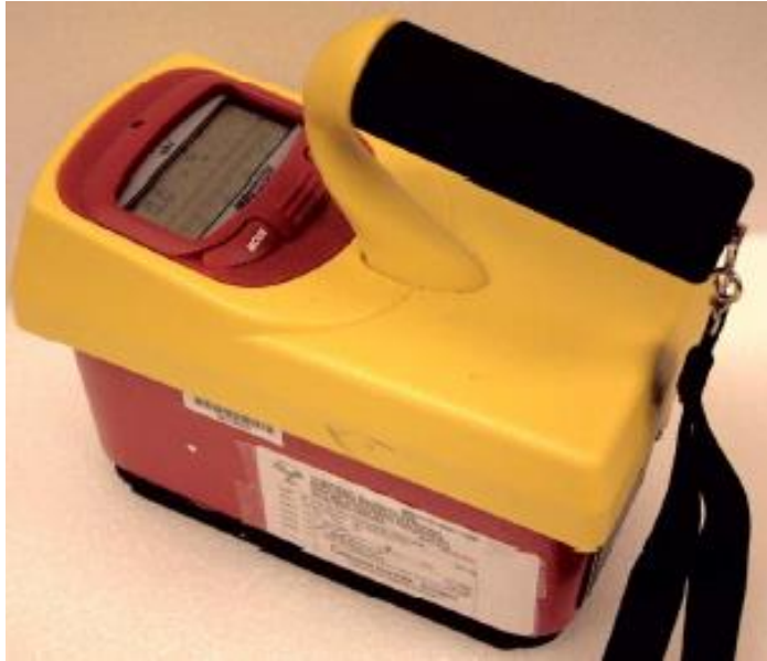
Fluke P451: Pressurized ion chamber very sensitive reads \mu\text{R}/\text{h} to \text{R}/\text{h} \mu\text{R} to \text{R}
