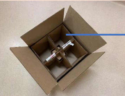
Pack the source in the approved carton using the same spacers / braces as in the incoming shipment.
