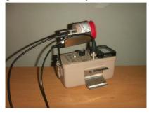
This instrument is used in the nuclear laboratory to detect radiation. There are usually at least two of these instruments at each site; an extra one is always available in case the other is found to be inoperable or needs to go out for repair or recalibration. There are regulatory requirements that must be followed concerning the use of these survey instruments:
